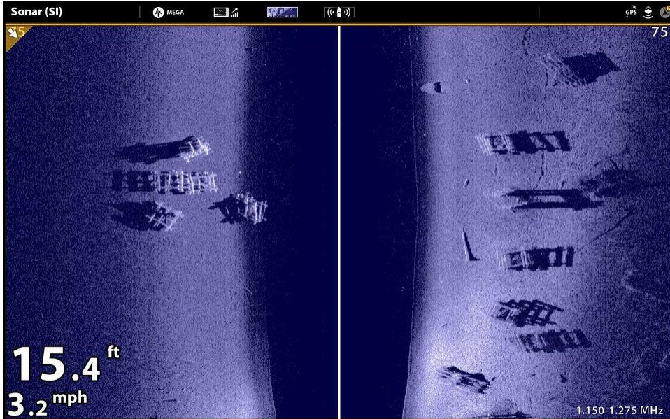
Figure 16: Example of the image resolution of the Humminbird Solix 15 Fish Finder in sidescan mode observing small fish aggregating devices in 15.4 feet of water depth (Image from a Humminbird brochure.)
