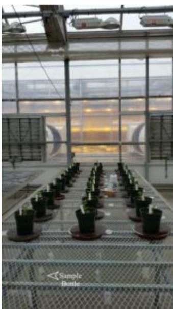
Phosphate sorption of leachate by coated sand was assessed by placing a tray of plain or coated sand beneath a pot planted with pansy, petunia, or chrysanthemum. Each tray was filled with 1 L (1,400g) of either plain or coated sand and covered with landscape fabric to prevent plant roots from colonizing the sand. Each tray had a drain that allowed the pot leachate to flow through the sand and drain to a sample bottle (Figure 1).
