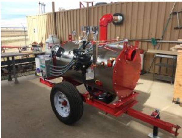
This steam generator is capable of steaming a 30'x50' section of growing bed to a depth of 2" in 2 hours.
