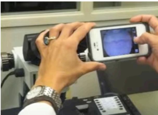
*Figure 1. Example of the Morrison Technique hand placement to stabilize a cell phone and capture a photograph through a microscope. Image Credit: YouTube Annie Morrison.*
