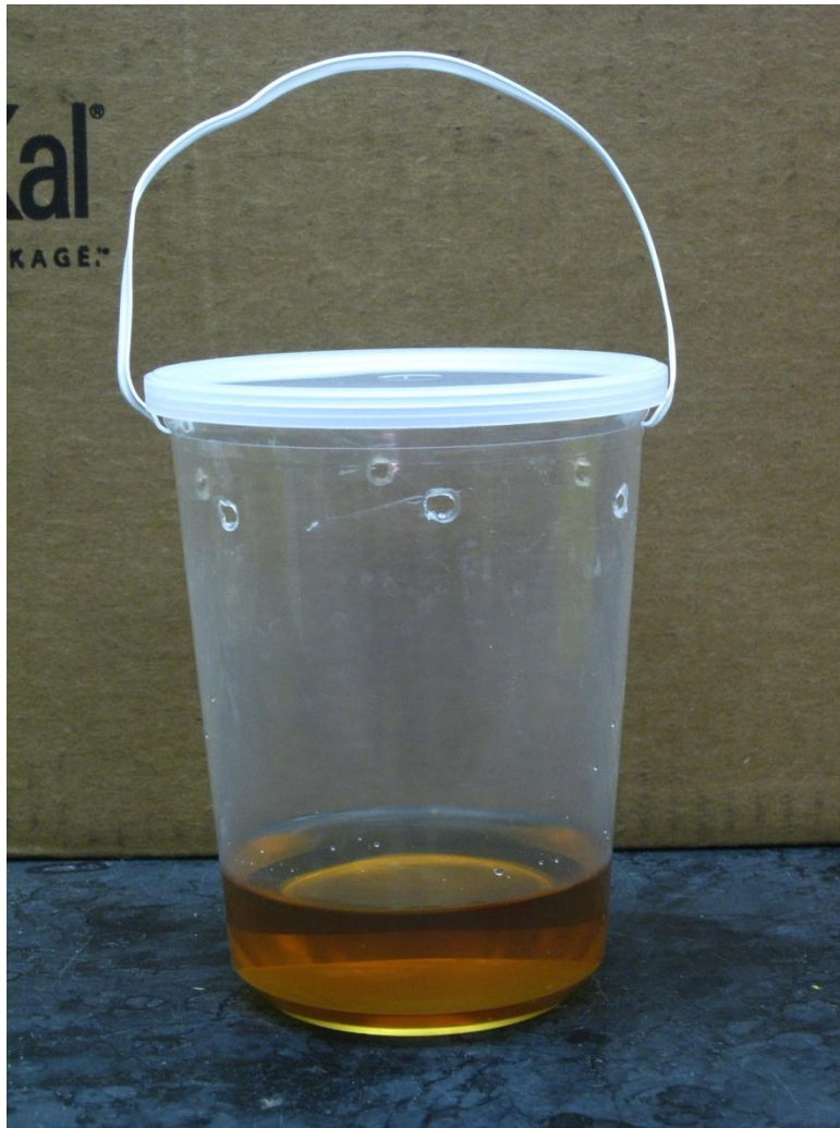
Figure 3-3. Plastic cup trap without yellow stimulus used for 2013 survey. Photo courtesy of L. E. Iglesias.
