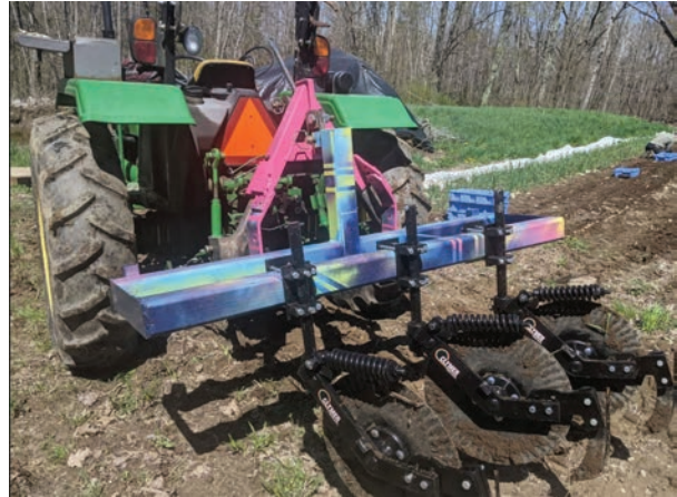
The coolest toolbar in the Northeast with 3 wavy coulters trailed by repurposed injector knives. This implement is pulled through tarped winter rye residue to improve transplanting of fall brassicas and cucurbit crops. Photo: Ryan Fitzbeauchamp.
