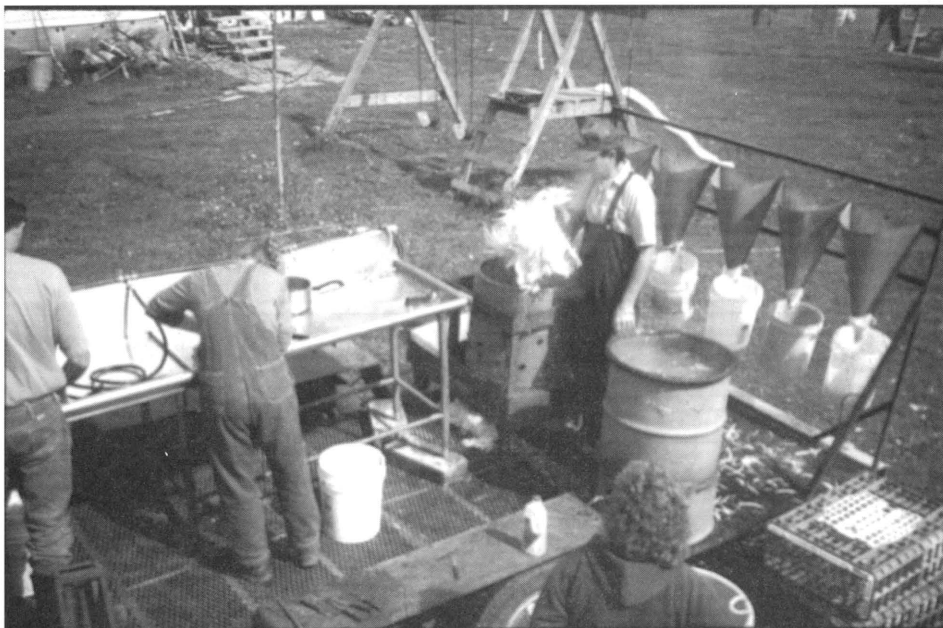
The Central New York Pasture Poultry Association's Mobile Processing Unit in operation. The man at right is standing between the scalding and plucking tanks, with kill cones behind him.
