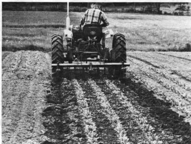
Dave Colson uses the Budding Basket Weeder for fine weed control in a young crop of spinach (see entry 13).
