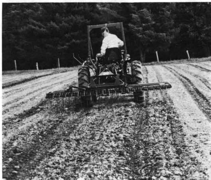
Mark Miller has demonstrated excellent weed control in strawberries with a Lely Springtine(see entry 44).
