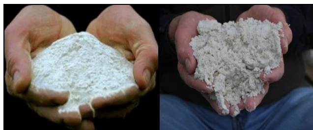
Figure 4. FGD gypsum (left) is white to light tan and has fine particles. Gypsum from other manufacturing processes (right) is greyish and, unless finely ground, tends to have larger particles (Source: www.gypsoil.com)
