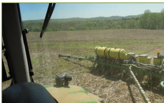
Fertilizer tanks filled with compost extract and injected in soil at corn planting
