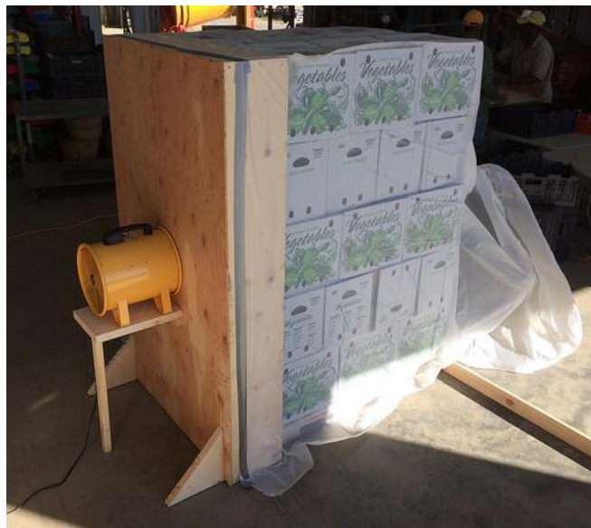
Figure 6 - Prototype forced air cooler setup for a pallet of stacked cartons. The fan is rated for 2520-2931 CFM at 2.1 IWC static pressure (Global Industrial, Model#T9F246343, $130). Typical required air flow rates for forced air cooling are 1-3 CFM per pound of produce at a static pressure of at least 0.5 IWC (Boyette, 1989).
