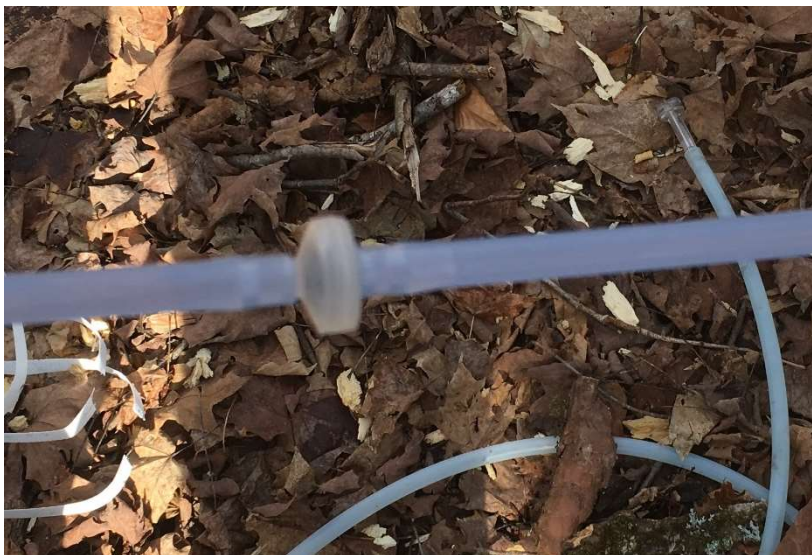
Picture of an inline 3/16" check valve (ILCK)
