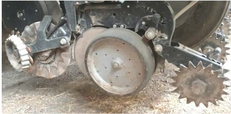
Figure 4. Properly adjusting row cleaners, row unit down pressure, placement depth, and closing wheel pressure will ensure stand established following a cover crop. These settings while important when planting into any conditions are more critical to ensure proper planting following cover crops.
