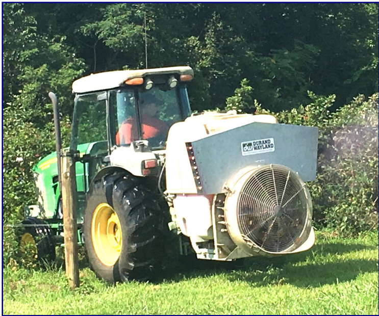
Figure 1. Airblast sprayer with a two-sided row crop head used in the 2018 blackberry trials.
