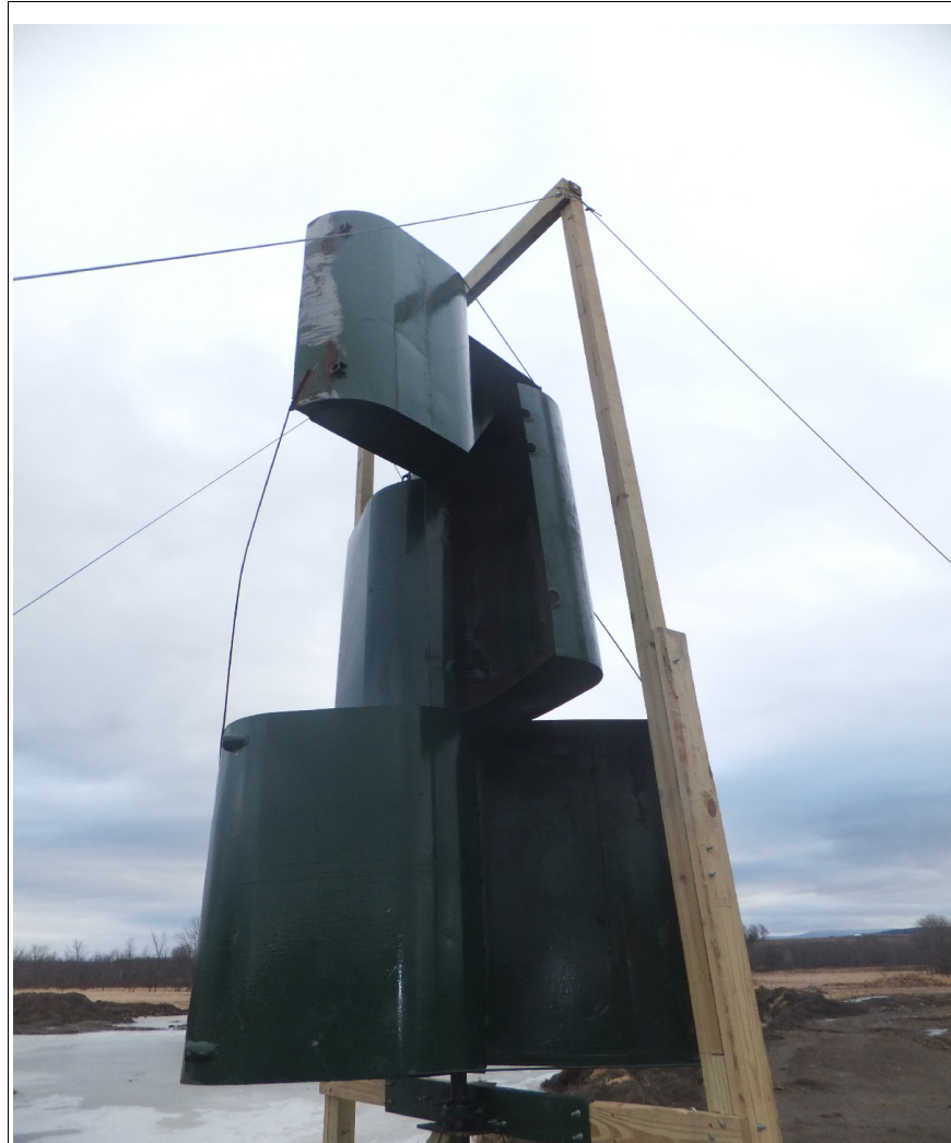
The finished product: A big green windmill. It's job beginning in the 2012 growing season will be to pump water from the reservoir (frozen water on the left) to the rice paddies (off to the right of the frame).
