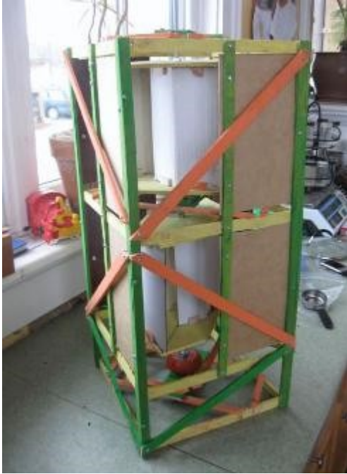
Illustration 1: 1/6th scale model of our "Mark I" Savonius built by Victor Gardy
