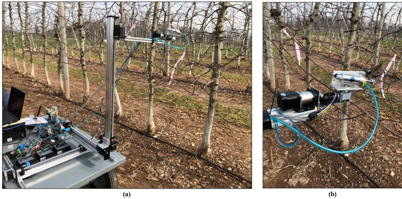
Figure 4. Robotic pruning system: (a) integration of end-effector with three linear actuators and (b) end-effector in use.
