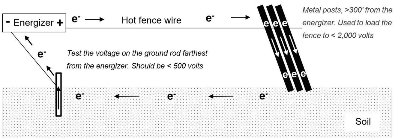
Figure 2. How to test a grounding system.
