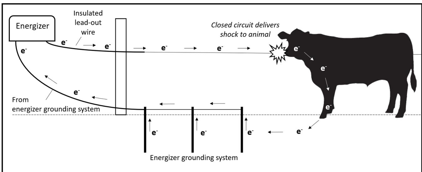
Figure 1. How an electric fence delivers a shock.
