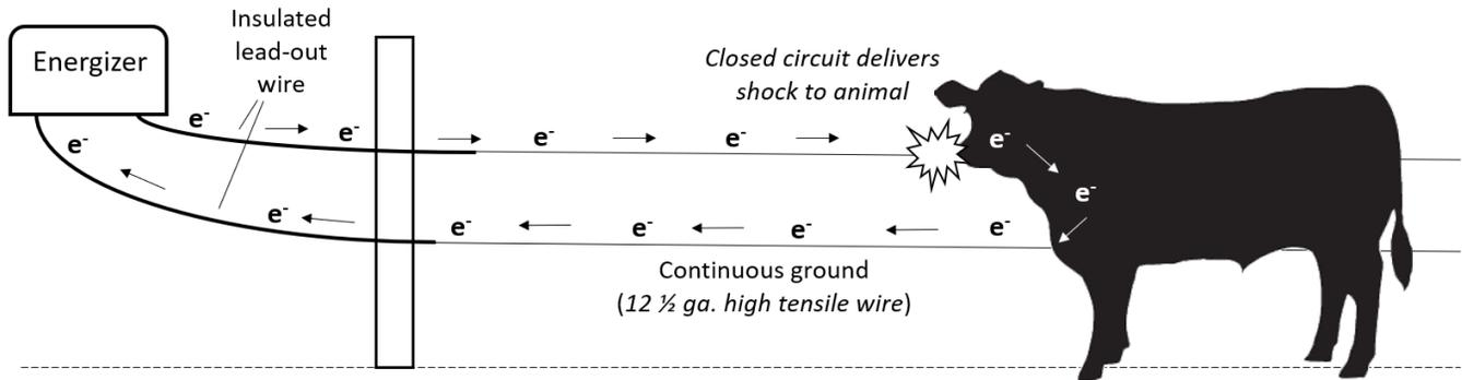
Figure 2. Continuous ground system.
