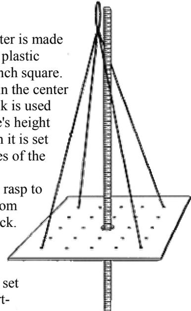
In addition 24, 0.125-inch holes are drilled along five lines set at 3-inch intervals, starting 3 inches from the plate's edge. Holes are spaced at 3-inch intervals along these lines, again starting 3 inches from the edge. This results in 24 holes (the 25th hole being in the yardstick hole). These holes can be used for estimating ground covered in thin stands and in grazed stubble.
