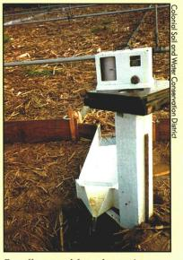
Runoff captured from the continuous no-till plot (above) was less in volume and contained less sediment and nutrients than the conventionally tilled plot (below).
