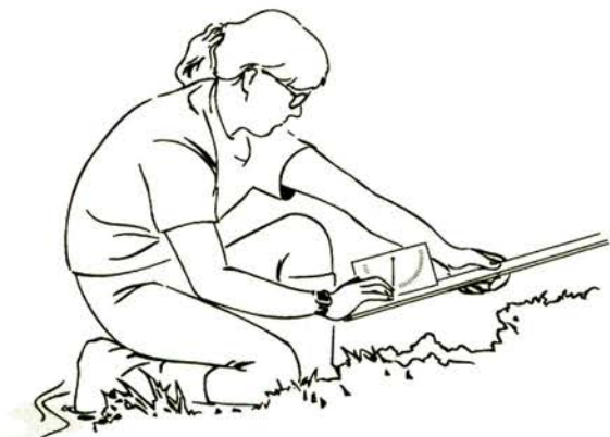
Figure 8a: Measuring bank angle with protractor and yardstick
