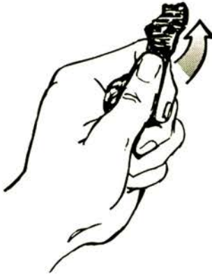
Figure 2: Assessing soil texture with the ribbon method
