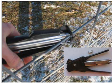
▲ Photo 3. The bottom 3-4 feet of the entire hoopie is covered with 1” chicken wire and fastened to the panels using wire or hog rings.
