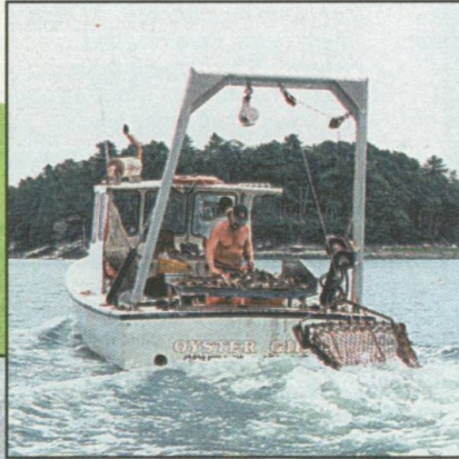
The company's vessel, Oyster Girl , is used both to disperse juvenile oysters on bottom for growout and for harvest. Below, partner Jeff McKeen with the dredge that is dragged on bottom to collect market-size oysters.
