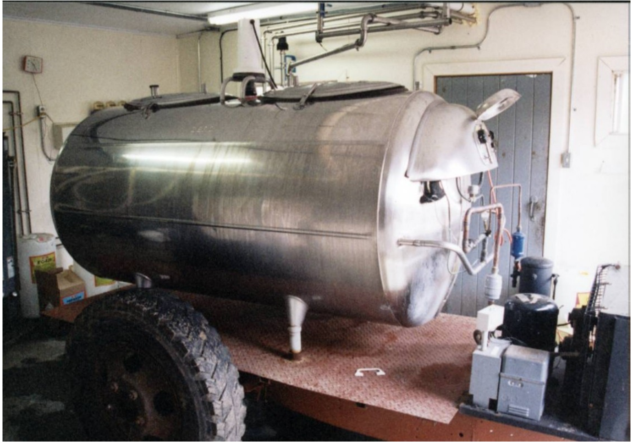
The tank is on wheels so that it can be hitched to a tractor and hauled to the cheese-making shed.
