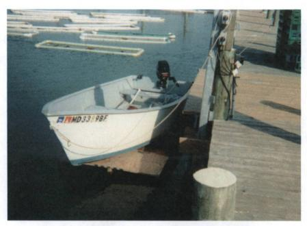
We gained out of water storage for a small boat. In this picture, the stern of the boat is floating while the bow is sitting high and dry. In this position the boat is easily boarded and floated off the platform. The skiff can be brought onto the lift much like it would be on a beach. The operator just steps out onto the lift and can then pull it up the rest of the way. He / she can then climb up onto the dock and use the lift to remove the skiff from the water. Because the arms
