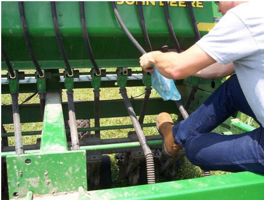
Calibrating no-till planter for dallisgrass + clover plantings (Objective 1)
