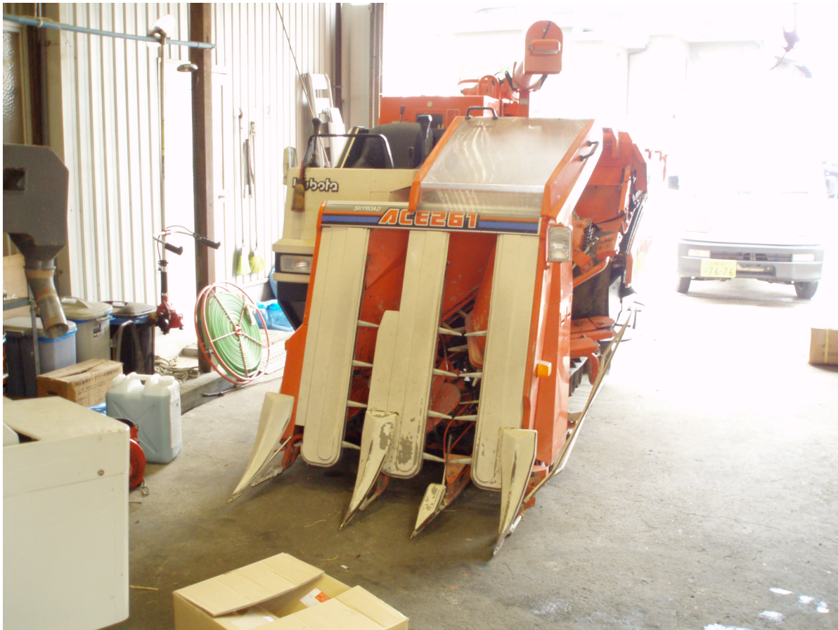
Photo 11. Rice harvester, which has a thrasher and caterpillar crawler (Gen Onishi).
