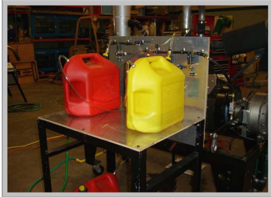
Figure 3. Fuel stand holds three 5-gallon fuel containers that are connected to the engine fuel system. Manual valves allow the operator to select the direction of the fuel flow between the experimental fuel, base fuel and flush fuel container.
