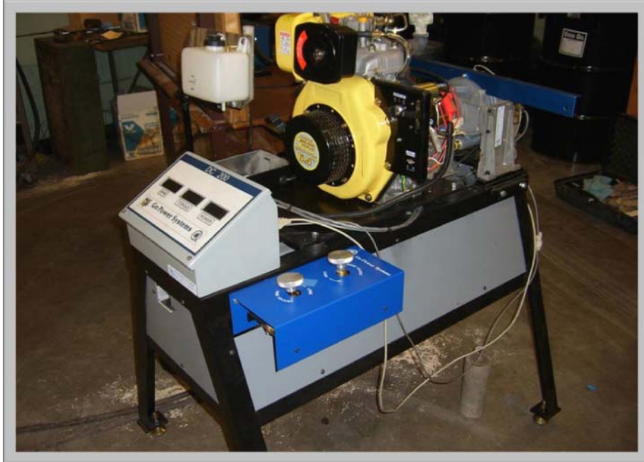
Figure 1. Single-cylinder 6.5 HP small diesel engine test stand. The frame, dynamometer and the engine performance monitoring system were available at the department. The single-cylinder diesel engine was purchased and mounted on the frame. Also two-fuel containers in 2-gallon capacity were mounted on the engine.
