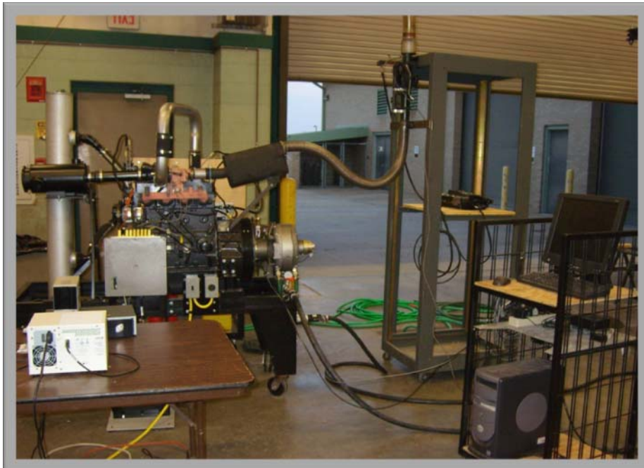
Figure 2. Cooling tower, 4-cylinder diesel engine, data acquisition terminal box, dynamometer, and the exhaust stand.
