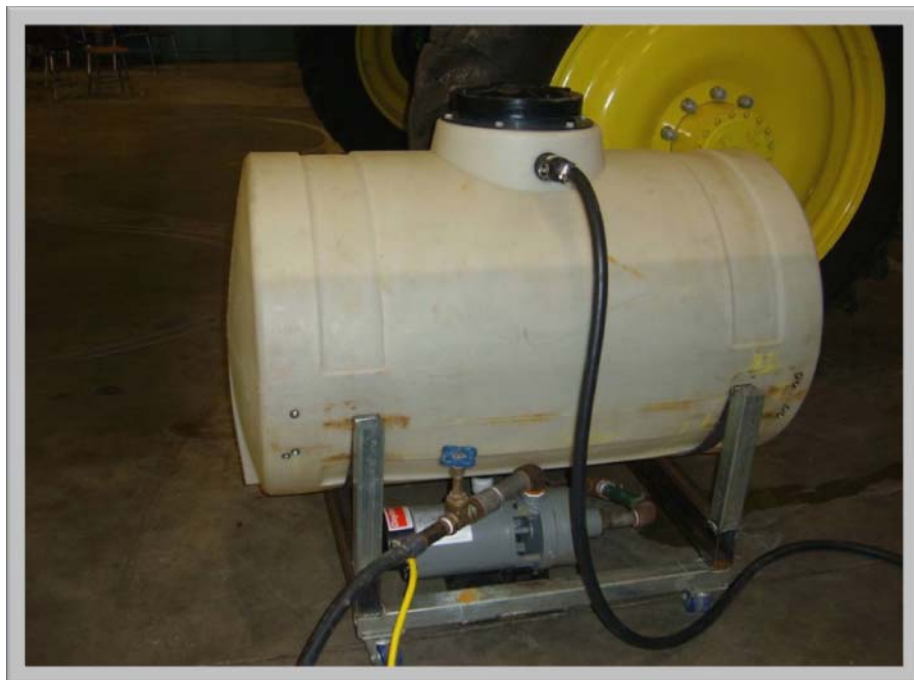
Figure 4. Water transfer tank with 200 gallon capacity. A frame on wheels was built to hold the water tank and the pump. The lower hose connected to the pump provides water from the tank to the dynamometer and the upper hose shows the water return line from the dynamometer.
