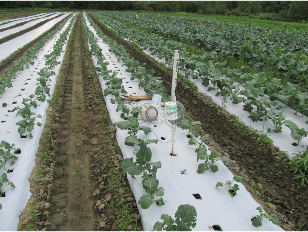
Thermal probes in Broccoli on plastic
