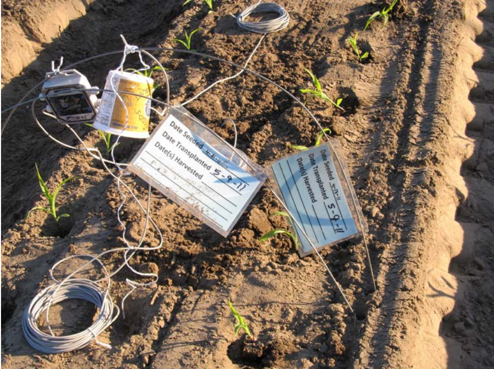
Air temperature 1 (lower) probe in Corn soon after transplant and initial setup. Note Datalogger as well.
