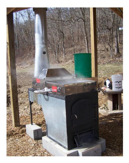
2x4' evaporator pan baffled rear pan shallow front pan
