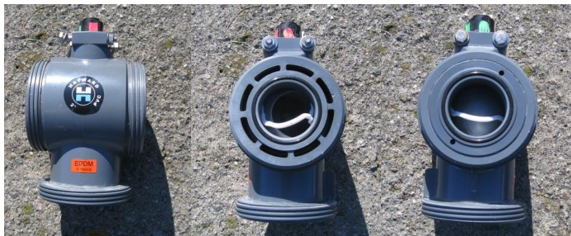
Fig. 2. Hayward valve that failed due to high heat.
