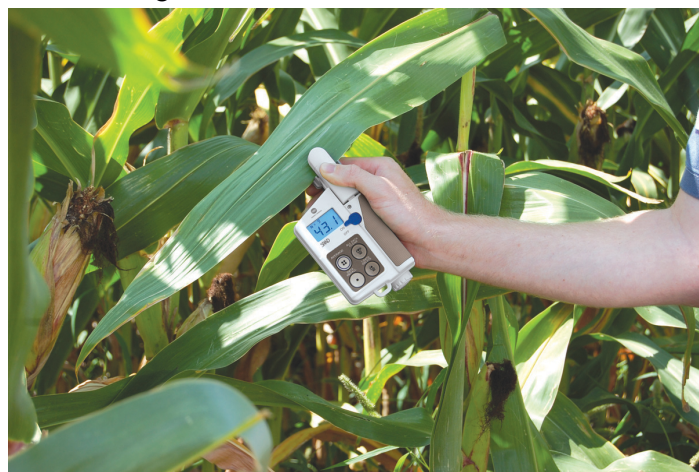
Konica Minolta SPAD-502 Plus chlorophyll meter
