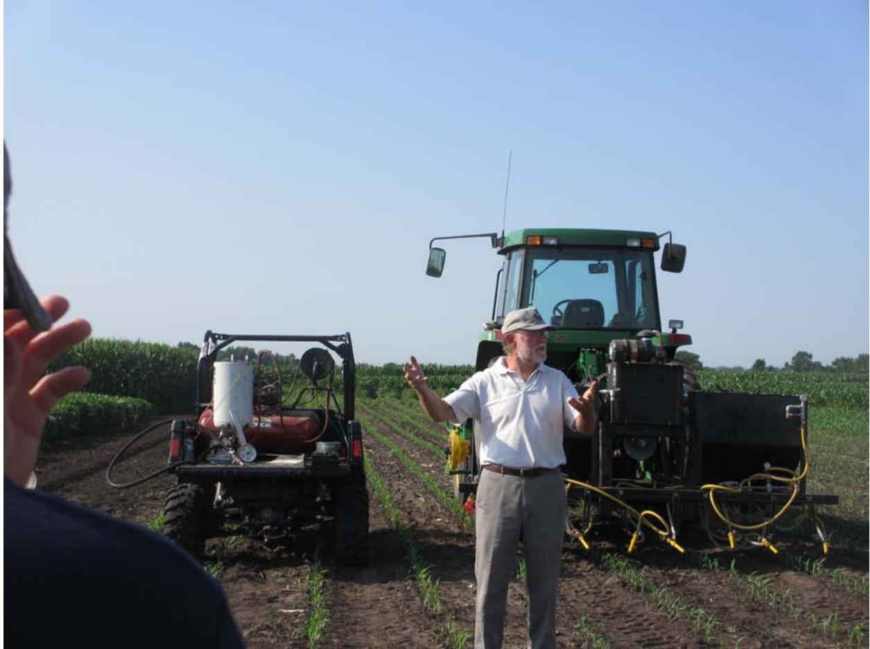
Figure 1. University of Minnesota Crop and Soil Field Day, July 2012. Tractor-mounted air-propelled abrasive grit applicator is shown to the right. Its construction had been completed only recently. Note the pairs of yellow nozzles, which are swiveled in several directions and ultimately aimed at the bases of the crop rows where small weed seedlings can be abraded by the emitted grit. To the left is the single-nozzle unit that was used for many preliminary experiments. The speaker is Frank Forcella.
