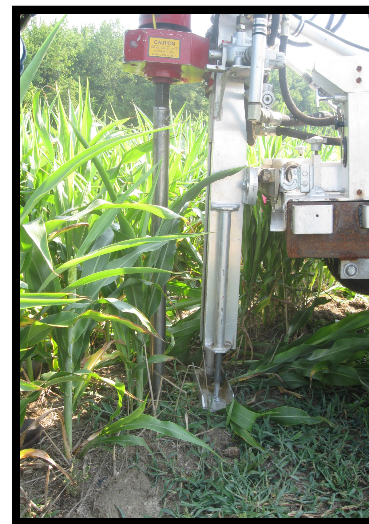
Figure 2. A hydraulic Giddings' probe was used to collect soil samples from the A and B horizons.
