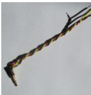
Twist the wires and make them look pretty (I like to first twist two and wrap additional wires one-by-one)
