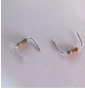
Two resistors to make a voltage divider. I used resistor values of  $R1=3.3k\Omega$  and  $R2=5.6k\Omega$  but plenty of other ratios will work (just be careful that you don't reduce current too much).
