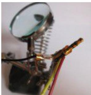
Finally add the ground wire to large metal tab
