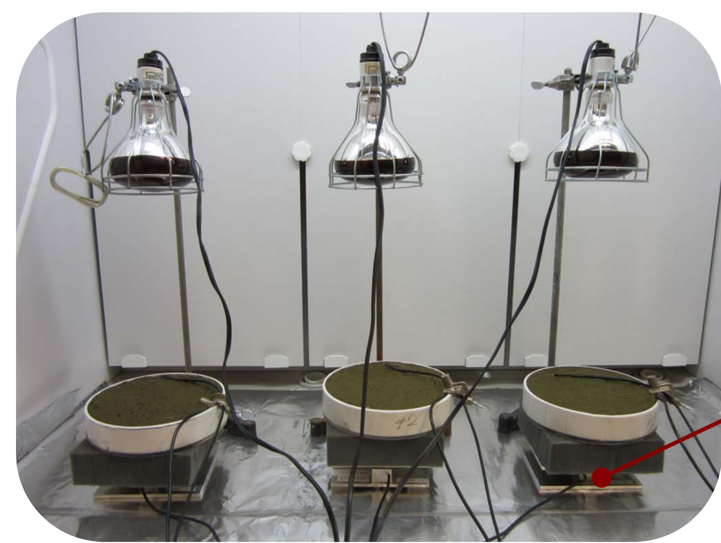
Pre-calibrated load cell (ESP-10, Transducer Techniques Inc., Temecula, CA)
