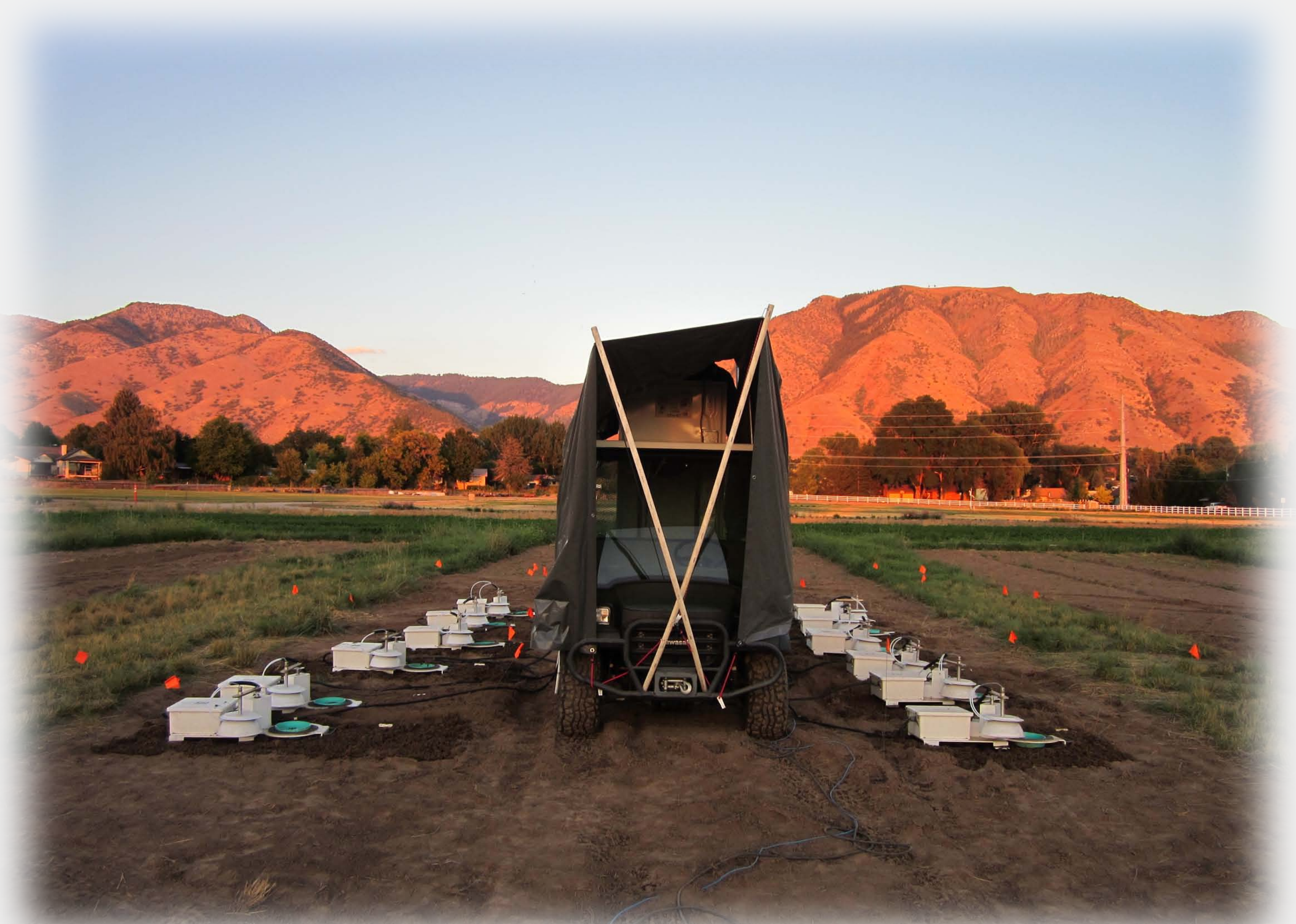
A multiplexed automated chamber system is employed for evaluation of manure management practices.
