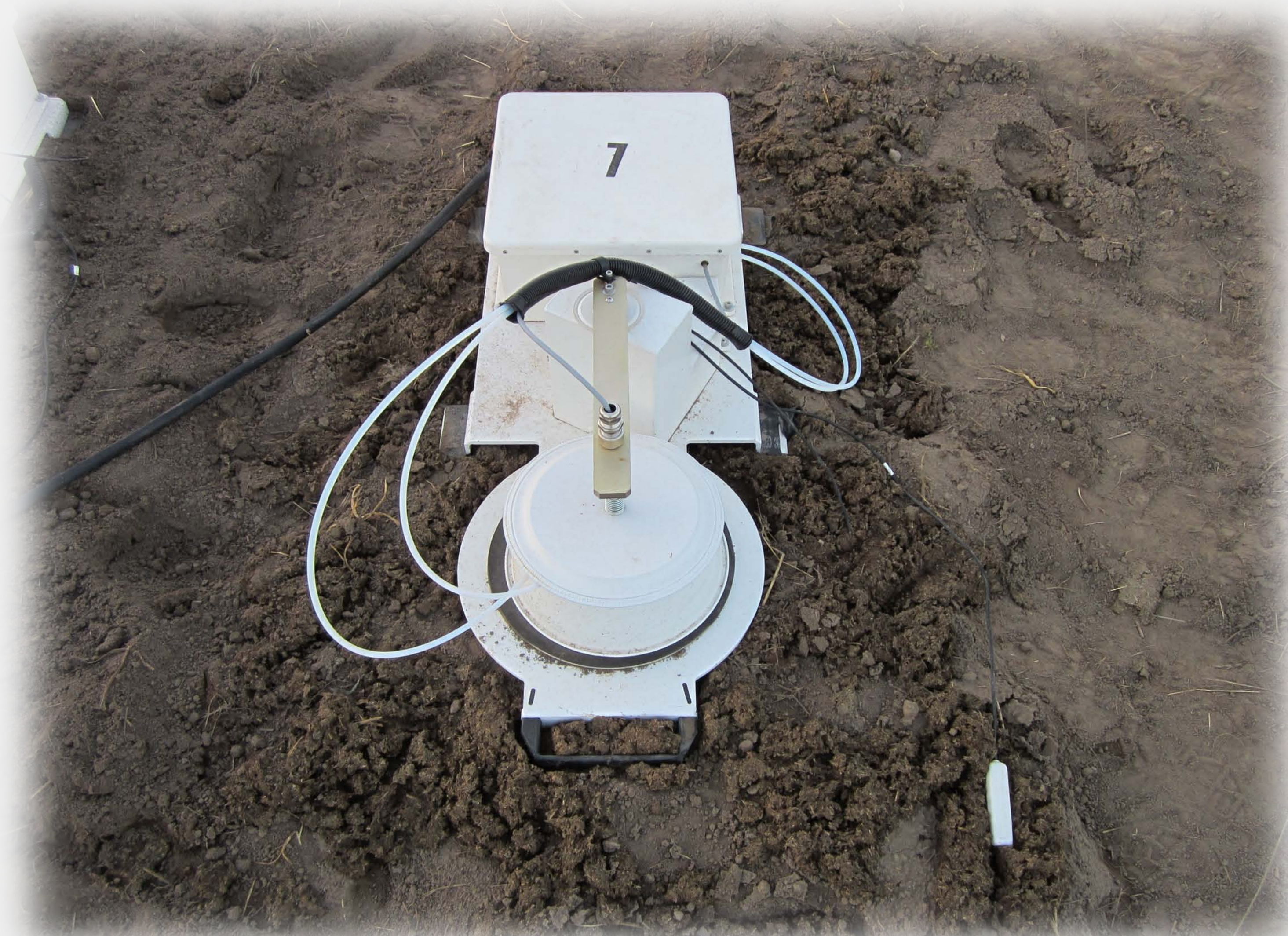
A closed dynamic chamber measures gas buildup to estimate emissions from soil surface-applied manure.
