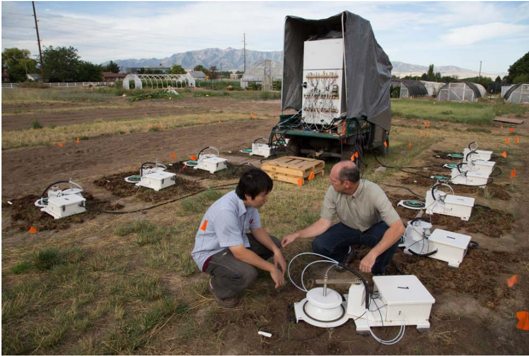
Figure 1. Field measurements carried out at the USU Greenville Research Farm in Summer 2013. In picture, the graduate student and his major advisor, Prof. Scott Jones, are inspecting the sensors and wiring installed in one of 12 chambers.
