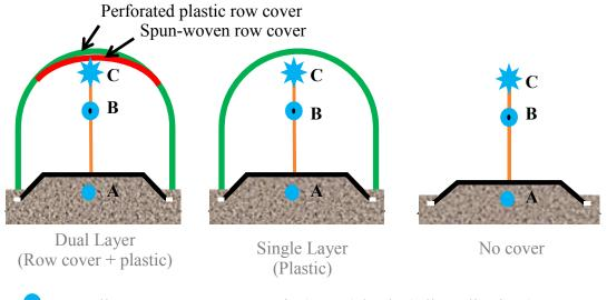
A: Soil temperature sensor at 4 in (10 cm)depth. (All Replications)
