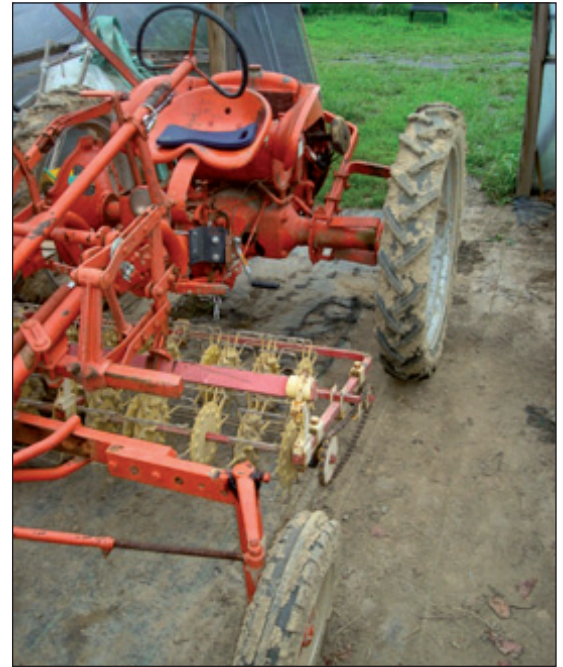
A basket weeder belly mounted to an Allis Chalmers G at Pennypack Farm and Education Center in Horsham, Pennsylvania. Photo: Andy Pressman, NCAT
