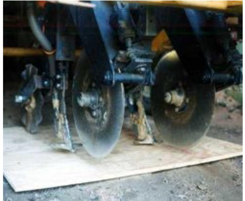
The front disk slices the residue, the shank (whose depth is adjustable) loosens the soil without inverting or incorporating the residues, the tube delivers organic fertilizer, and the fluted coultter mixes it into the planting slot. A no-till transplanter with specially-designed press wheels then places seedlings or seed potatoes into the slot.
