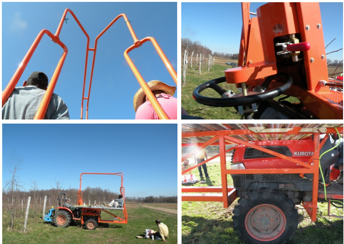
Figure 1. A 7 ft. x 9 ft. platform mounted over the hood of a tractor from which two workers can prune adjacent trellis walls. Notice the self-steering mechanism incorporated with the platform.
