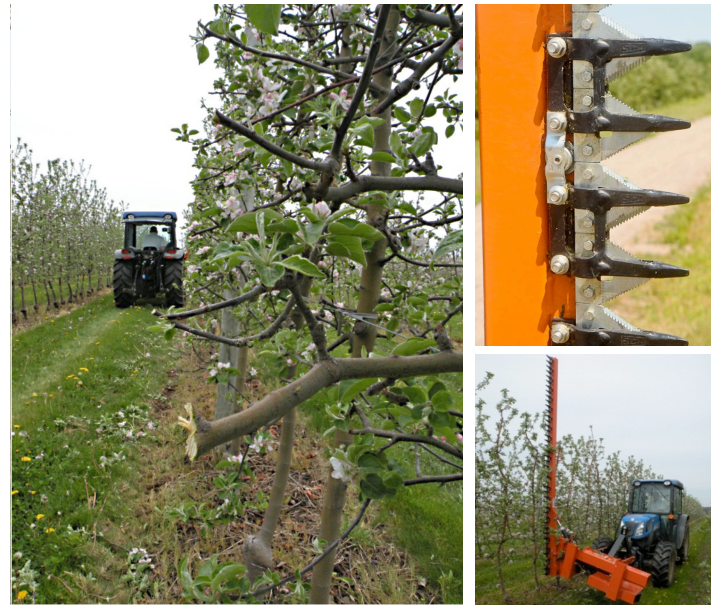
Figure 4. With a Super Spindle tree and 10-11 ft. row spacing the hedging is done one ft. from the trunk (the fruit wall is very narrow).
