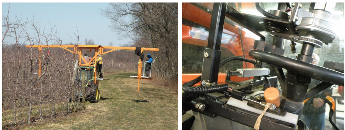
Figure 2. A 7 ft. x 9 ft. platform mounted over the hood of a tractor from which two workers can prune adjacent trellis walls. It has two additional 4 ft. x 5 ft. outboard platforms suspended from booms, which can be swung out over the adjacent rows. Each of the over-the-row platforms carries a single worker.
