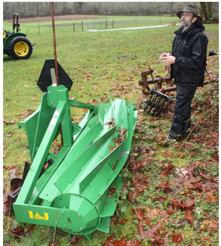
Figure 1. Jim Meyer, Cascadian Home Farm manager, and his roller/crimper from I&J Manufacturing. Photo credit WSU.
