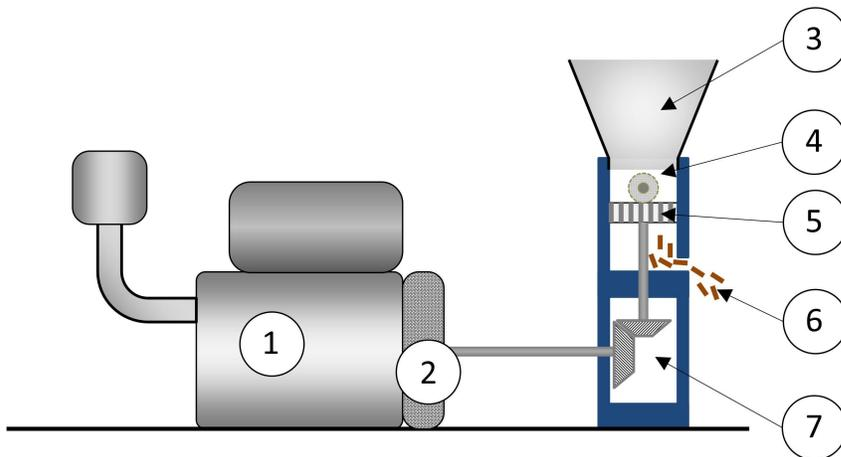
1 – Diesel engine, 2 – Clutch, 3 – Infeed hopper, 4 – Rollers, 5 – Die, 6 – Pellets exiting pelletizer, 7 – Gear box
