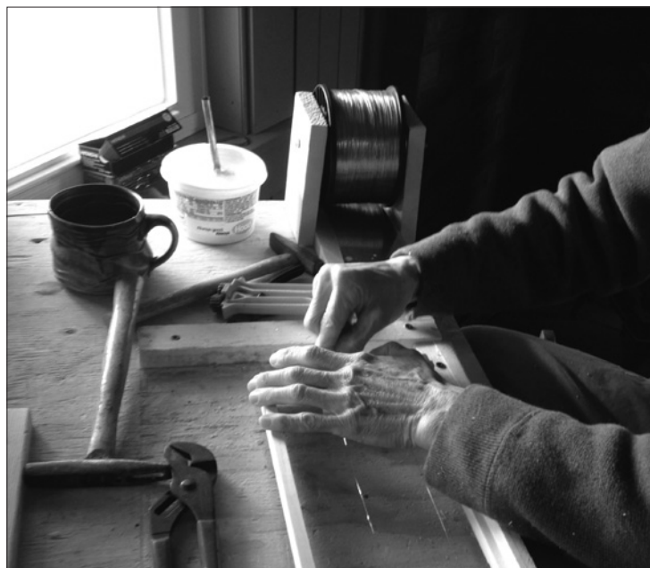
She cross-wires the frame, crimping the wire afterward (not depicted, but see the crimping tool just beyond her right hand).
