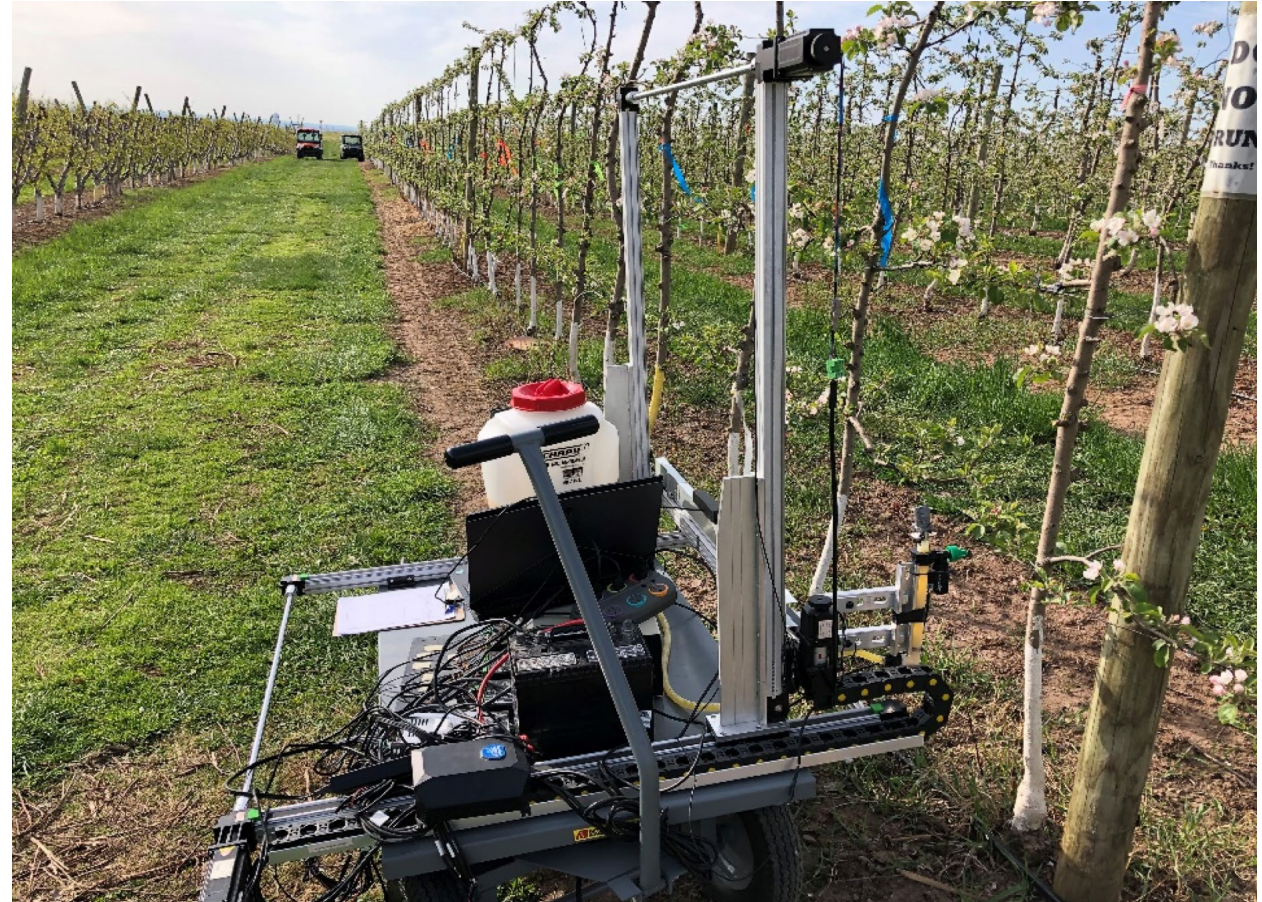
Cartesian target spraying system developed in 2022
