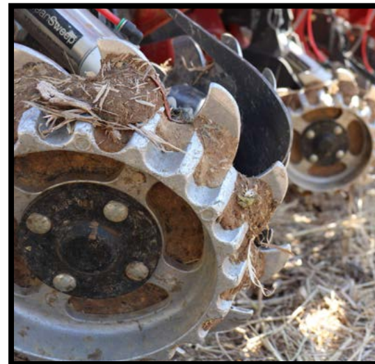
Shark tooth row cleaners with depth bands are very effective in thick residues.
