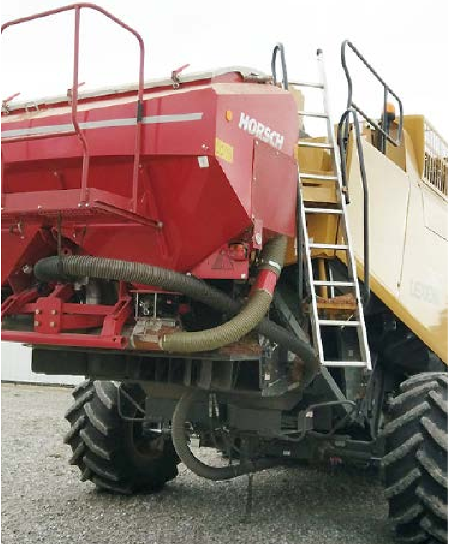
Horsch seeder hopper feeds air-driven seed to distribution outlets spaced for uniform delivery under combine header.
