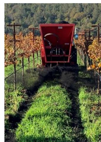
Photo 1. Applying biochar with mulch spreader.
