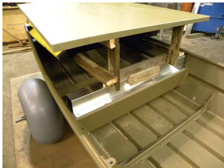
Frame standoffs to allow for table connections.
