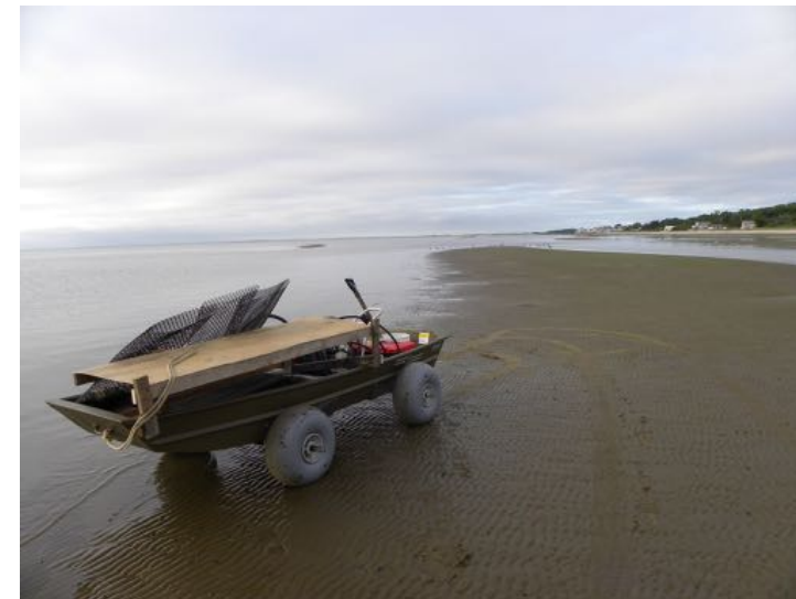
Field test with modified axle/wheel turning radius.
