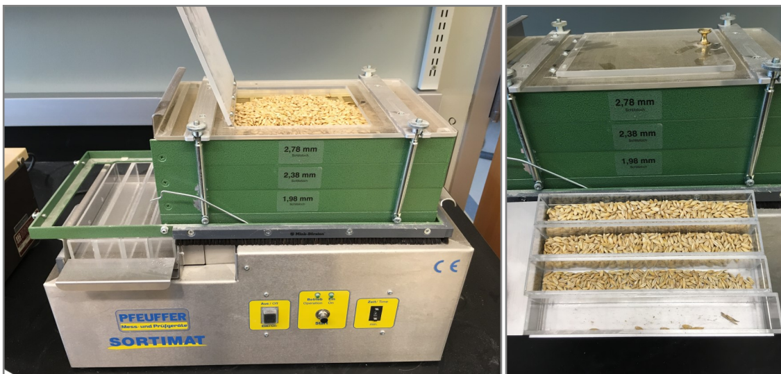
Image 1. Barley being sorted for plumpness at NWCS Quality Testing Laboratory, Burlington, Vermont.
