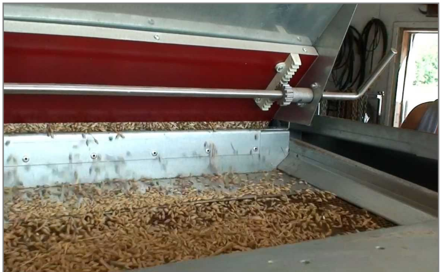
Image 10. Barley being cleaned with a screen cleaner.
